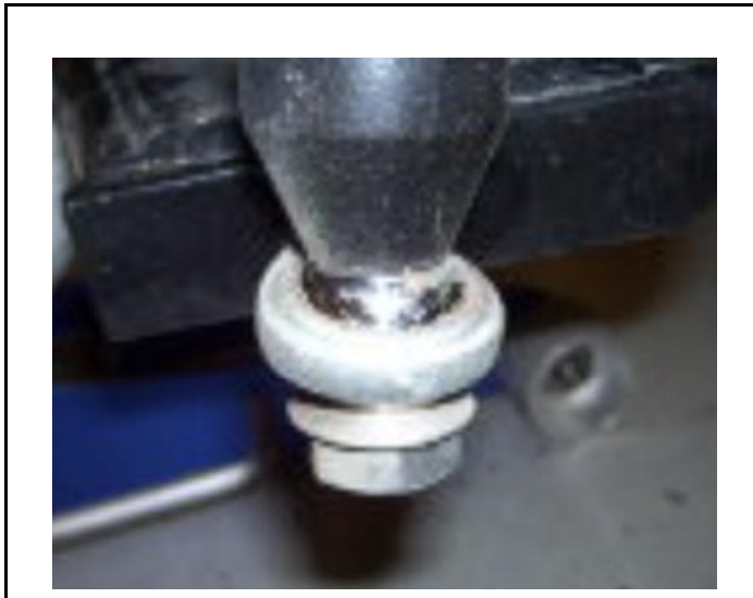
Figure 7-12 Correct orientation of rod end to ball
